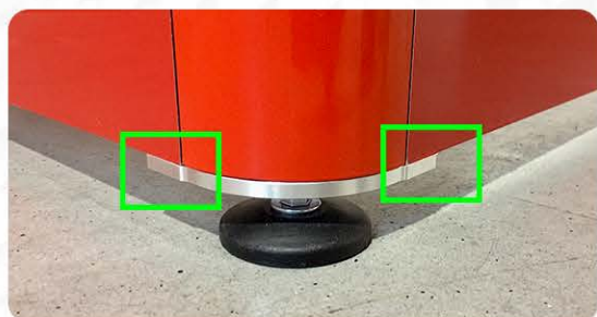
INSERTION BUFFER ISLANDS FOR PANEL
